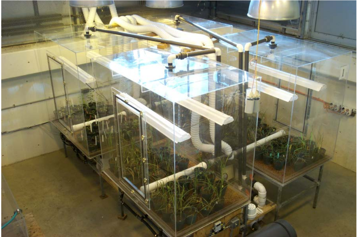
Figure 1. A 4-chamber, greenhouse-based CO 2 exposure system was constructed at the Alberta Research Council, Vegreville, Alberta to conduct studies on the effects of elevated CO 2 on crops and weeds.
